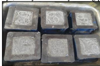
Figure 3.1 Casted mortar cubes
