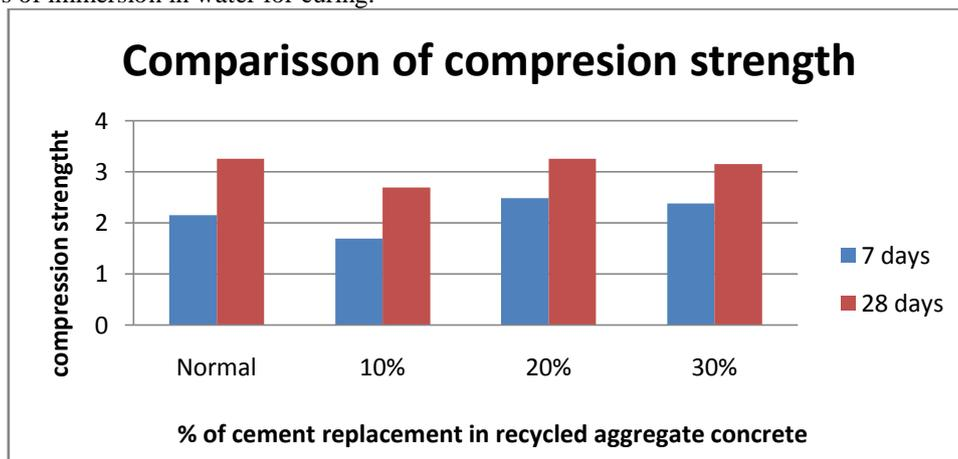
The compression strength of concrete increases with recycled aggregate concrete with 20% replacement of cement by using fly ash.
