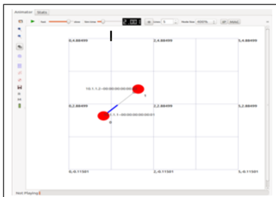
Fig.2- Nodes linking through point to point link in NetAnim
