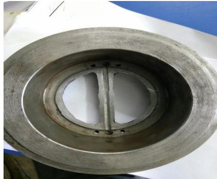
Fig. 5- Dual plate check valve after machining
