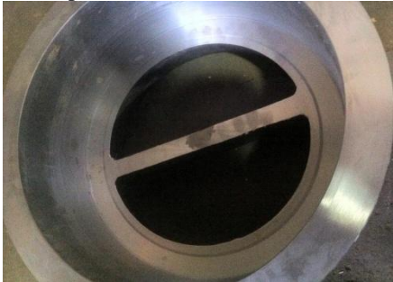
Fig. 2- Dual plate check valve before welding
